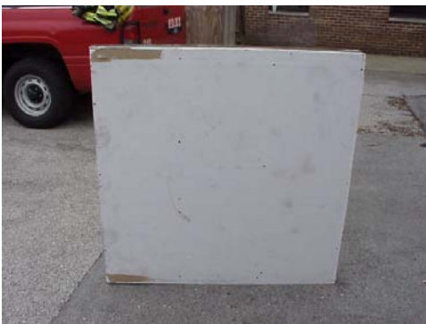
4' x 4' wall with metal stud framing and Hi-Impact 8000 wallboard mounted to both sides of the wall.
