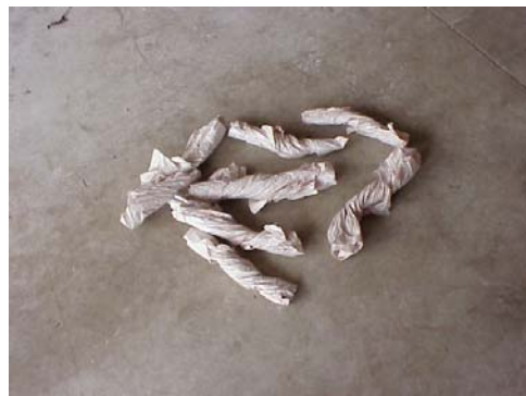
Approximately 4 pieces of white packing paper were ignited inside the wall to simulate burning materials that have dropped into the wall during a structure fire.
